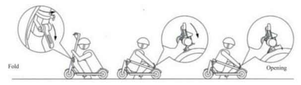
Make sure the scooter is turned off before folding. Open the folding mechanism on the handlebar and fold the handlebars. Secure the handlebars to the buckle on the rear fender.
