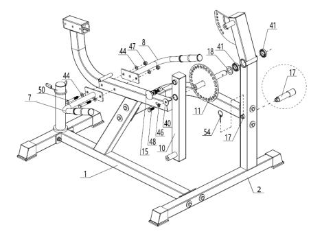
Fix the backrest frame (5) to the main frame (1) with bolts  $M10^{*}25$  (48), washer (44) and M10 hand knob (47)
